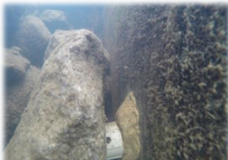
Figure 3. Cobble leaning on PVC housing to ensure that the epoxy sets.
