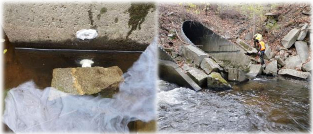
Figure 4. Photo A depicts the metal tag and PVC housing. Photo B gives a wide view of the site.
