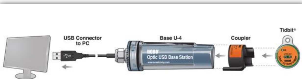
Figure 2. Diagram illustrating the use of a base station for downloading logger data.
