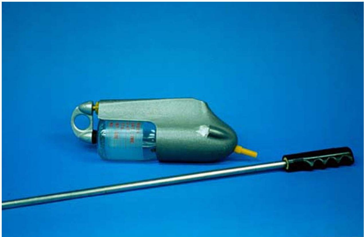
Figure 4. DH-48 depth integrated water sampler for collecting suspended sediment samples. Handle (partly shown at bottom) attaches to top of metal housing when in use.
