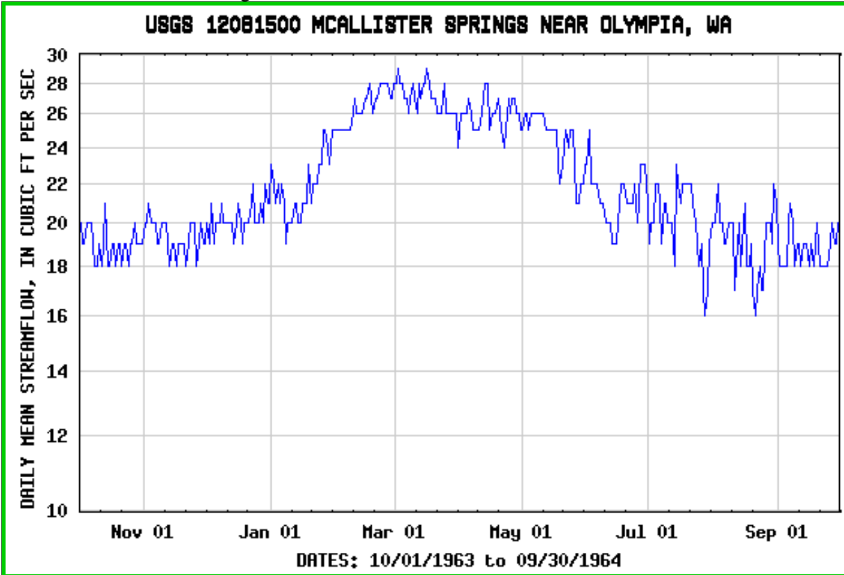
Figure 9. Groundwater-dominant hydrograph, 1963-1964, McAllister Springs. Source: USGS. Water Resources of Washington 7
