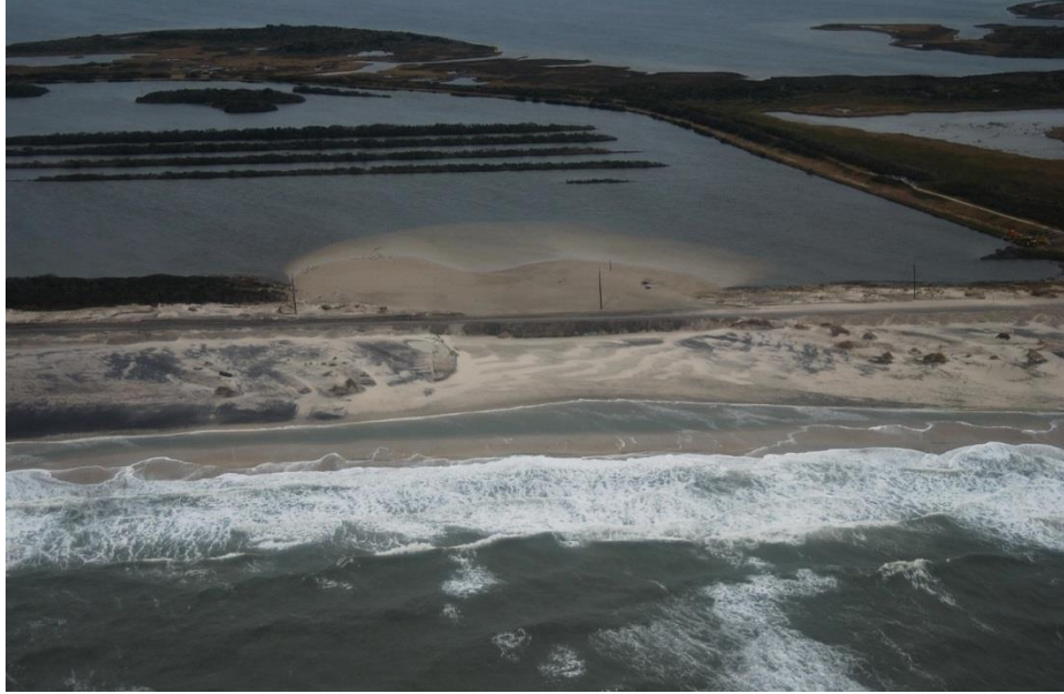
Figure 7. Overwash breached the dunes protecting North Carolina Highway 12 (NC 12) at Pea Island NWR in North Carolina, crossing the roadway and depositing an overwash fan in one of the refuge's impoundments. In this USGS (2015) image from November 6, 2012, the NC Department of Transportation has already removed the overwash from the roadway and piled the sediment on the beach as an artificial dune.
