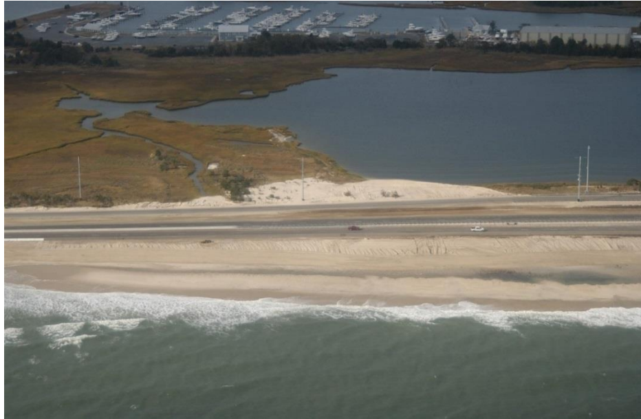
Figure 3. Overwash occurred in limited areas in Delaware, most notably north of Indian River Inlet in Delaware Seashore State Park. Nearly all of the overwash deposits were scraped back onto the beach to form artificial dunes within one week of the storm, as seen in this image from near the Indian River Marina where the overwash extended across both roadways on the barrier spit to the bayside. Image from USGS (2015) dated November 6, 2012.
