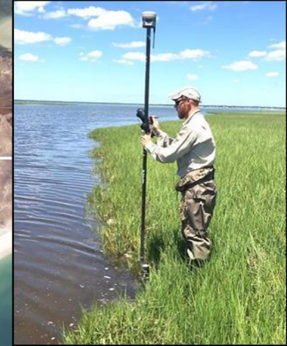
Surveying Water Level Logger to relate local tidal datums with the marsh surface
