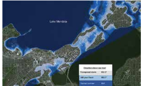
A case study transposed historic storm data to near Madison, WI, resulting in overland flows and urban runoff that would swell streams to new heights, Lake Mendota (shown here) overflowing its banks, the closure of the regional airport, and the City of Madison being split in half by floodwaters that could remain standing for as long as ten days. (Figure: Daniel Fletcher)
